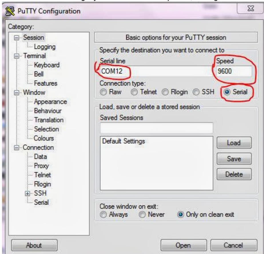
Dans le menu Category / Serial/ paramétrer Serial line to connect = COM12, speed = 9600 baud, data bits=8, stop bit=1, parity=none, Flow Xi=on/Xoff.
