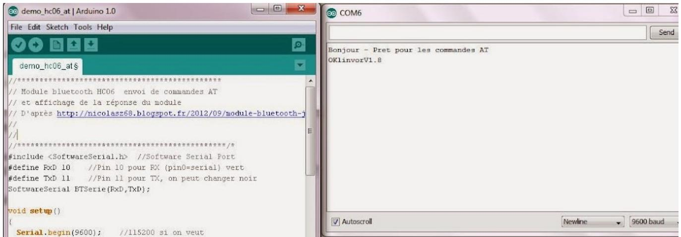
The screenshot shows the Arduino IDE with a sketch named 'demo\_hc06\_at' open in the editor. The code is a simple AT command example for the HC-06 module. The Serial Monitor window shows the module's response to the AT command.
